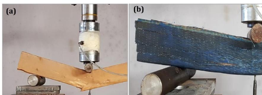
**Figure 6.** Failure modes (a) unreinforced beam, and (b) reinforced beam.
