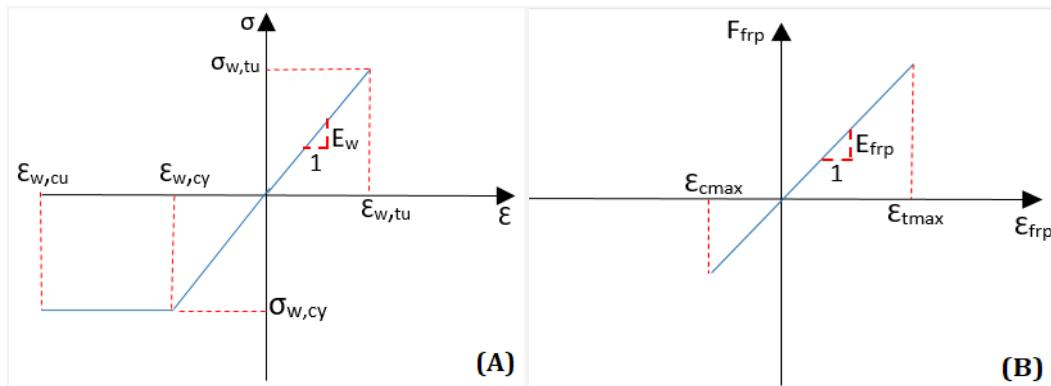
**Figure 4.** Constitutive law for (A) wood, and (B) fiber reinforced polymer.
