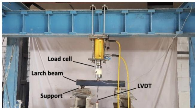
Figure 3. Real image of the bending test experimental setup.
