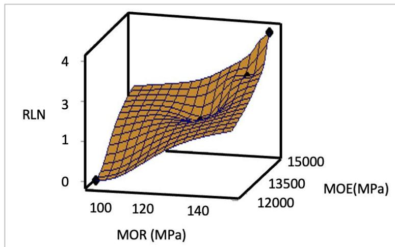
**Figure 10.** Modulus of rupture and modulus of elasticity values depending on the number of FRP layer (3D graph).
