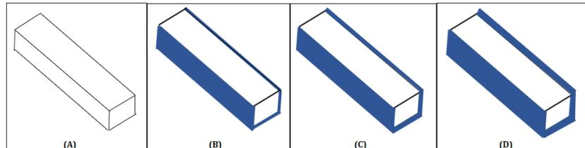
**Figure 1.** Schematic view of beams (A): Reference beam, (B): 1-layer reinforced beam, (C): 2-layer reinforced beam, and (D): 3-layer reinforced beam.
