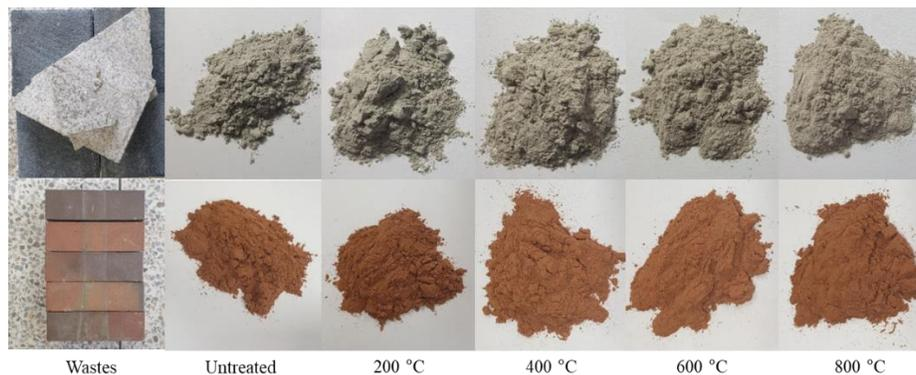
**Figure 4.** Granite and clay powders at elevated temperatures.
